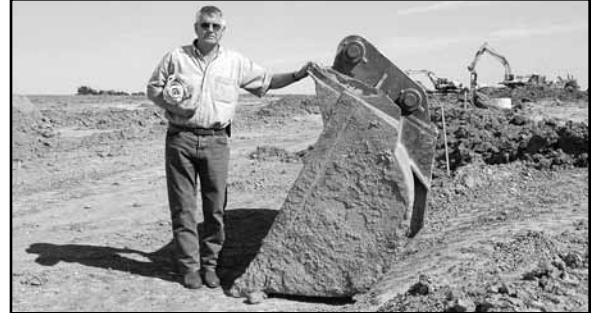
Larry Roloff and L.G. Roloff Construction Company have been innovators in the construction industry in Nebraska. Here he stands next to a bucket that was fabricated by his company to incorporate a modified hitch for a quick coupler.
