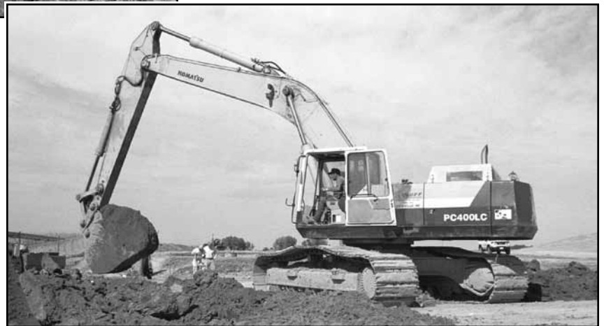
Larry Roloff and L.G. Roloff Construction Company have been innovators in the construction industry in Nebraska. Here he stands next to a bucket that was fabricated by his company to incorporate a modified hitch for a quick coupler.
